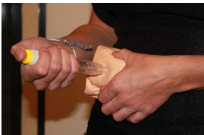
Fig. 12 Simulated subcutaneous injections were performed in a foam pad, mimicking skin behavior [43]. The release button can be activated only if the system is pressed well to the injection site (Photo reproduced with permission from Becton-Dickinson)
