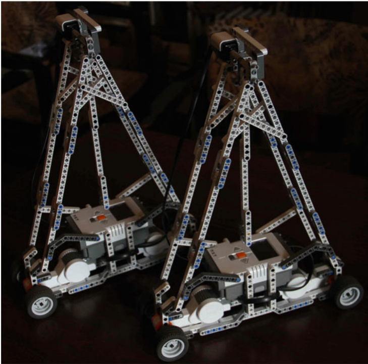
Fig. 5 Two similar pendulums on cart constructed with Lego Mindstorms NXT
