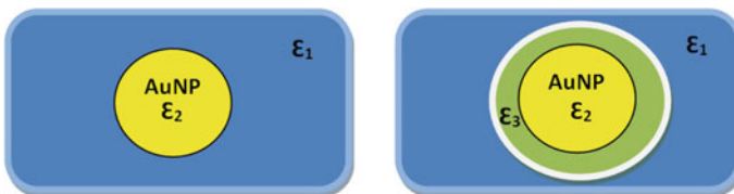
Fig. 6 Methodology for modelling coated and non-coated metallic nanoparticles in MNPBEM Matlab toolbox
