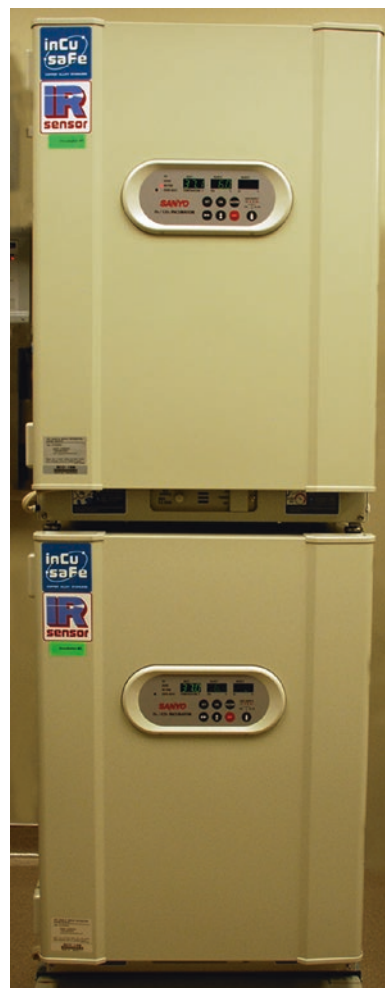
■ Fig. 10.2 A 170 L infrared CO 2 sensor, conventional air-jacketed incubator. Faster CO 2 recovery can be expected with a large infrared sensor-equipped incubator than with a smaller incubator with a thermoconductivity CO 2 sensor
