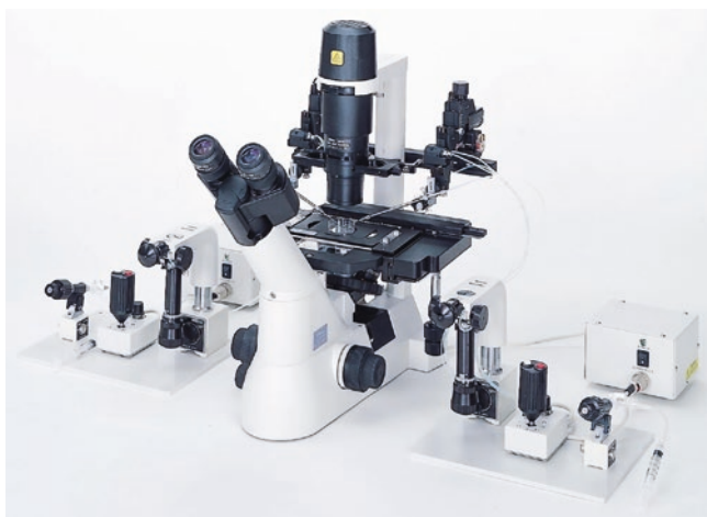
■ Fig. 35.1 Example of setup for ICSI with electrical coarse manipulators and hydraulic manipulators for fine movements. (Courtesy of Nikon, Melville, NY, USA)
