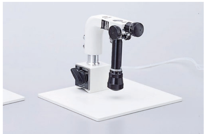
■ Fig. 35.2 Example of control unit of hydraulic manipulator with hanging joystick. (Courtesy of Nikon, Melville, NY, USA)
