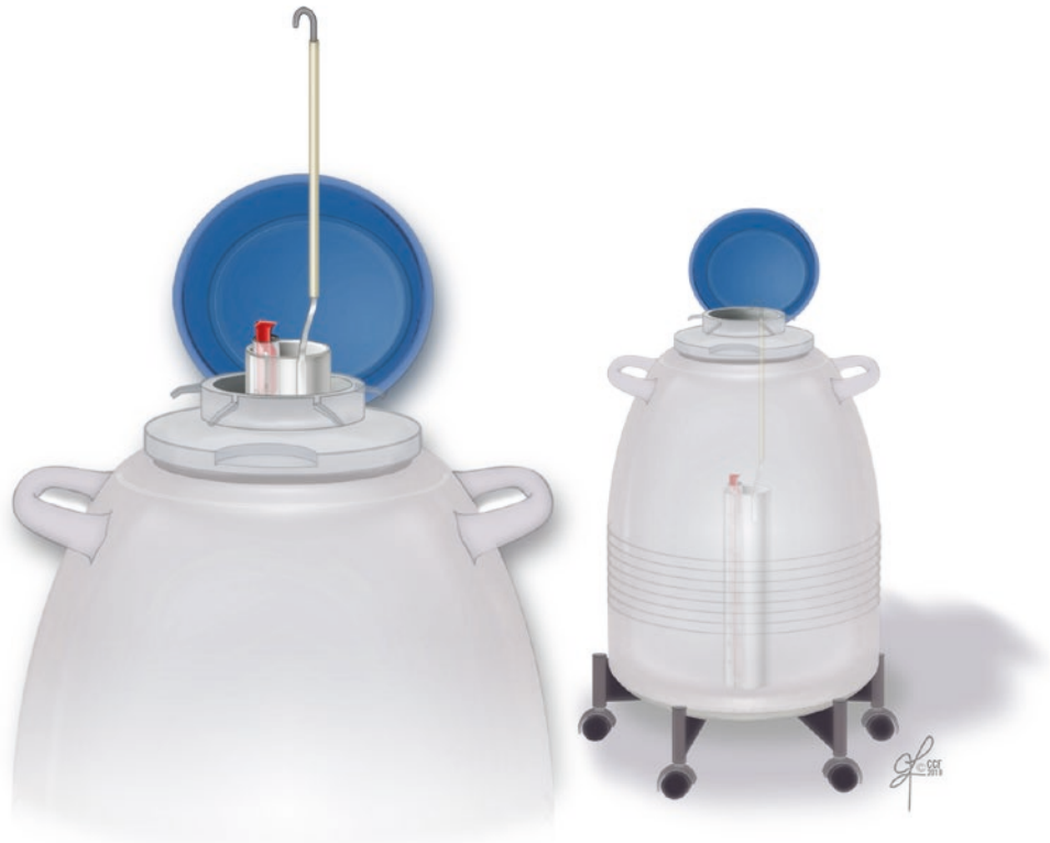
■ Fig. 51.5 The cryovials should be placed into the cryocanes before immersion in liquid nitrogen vapors
