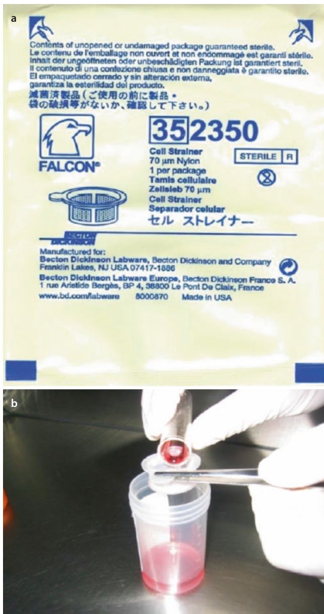
■ Fig. 17.1 a Labeling on Cell Strainer (Falcon, Becton Dickinson and Company, USA); b follicular aspirates are filtered with a Cell Strainer
