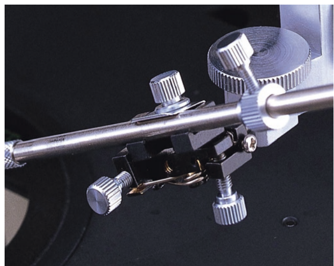
■ Fig. 35.6 Example of a more recent type of universal joint where changes in position can be made by simple rotation of screws with mounted tool holder. (Courtesy of Nikon, Melville, NY, USA)
