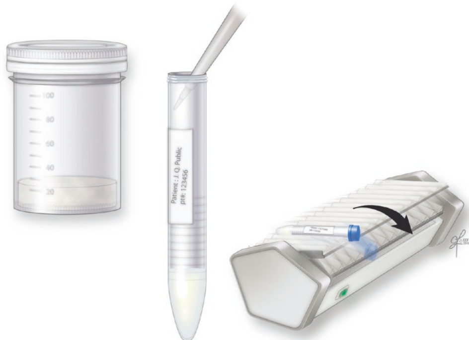
■ Fig. 51.2 A volume of TEST-yolk buffer at 37 °C, equal to 1/4 of the sample volume should be added, then the specimen plus the TEST-yolk buffer is gently rocked for 5 min
