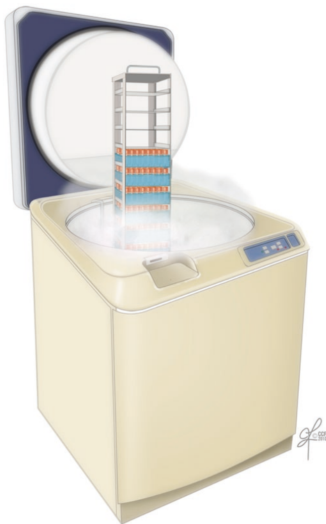
■ Fig. 51.7 Vapor phase step in the cryopreservation by slow-freezing process
