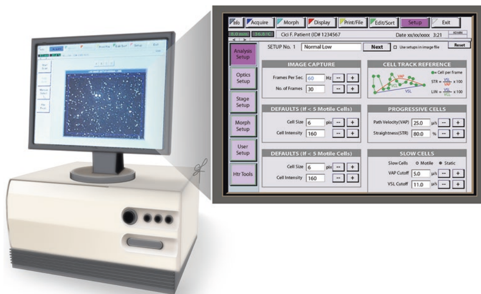
Fig. 22.5 Representative image of a computer-assisted semen analysis (CASA) system and display of the obtained results
