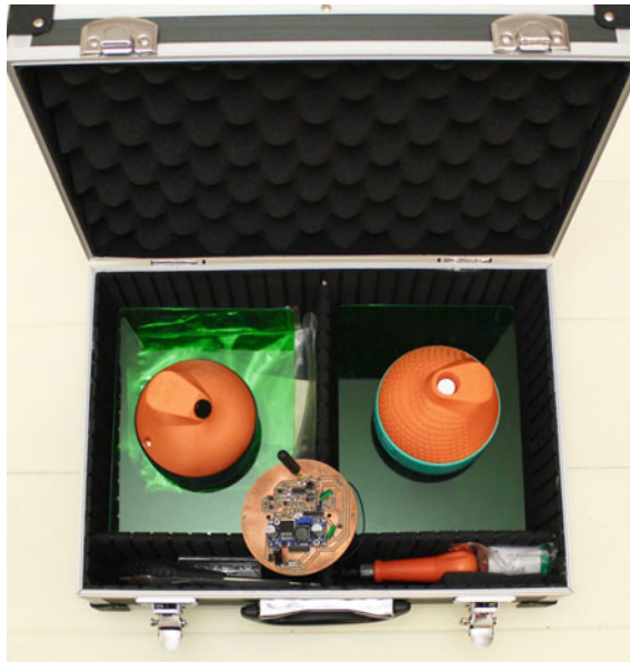
Fig. 6 Autonomous garbage level sensor unit—2 design variants
