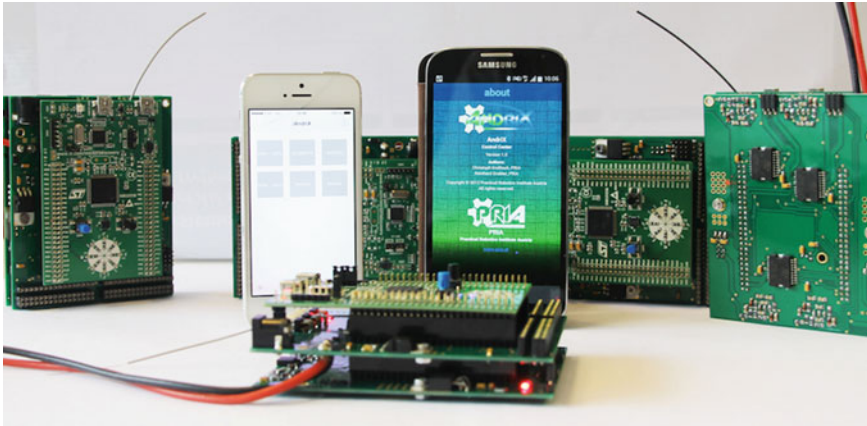
Fig. 2 Robotics controller Hedgehog and according smartphone app for programming and controlling robots
