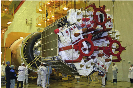
Fig. 8.22 Integration of three GLONASS-M satellites with a Block-DM upper stage (courtesy of ISS Reshetnev)
