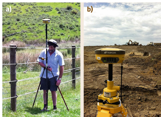
Fig. 35.9a,b Establishing coordinates of control marks using GNSS: (a) setting up a GNSS receiver/antenna set up over rural control mark using a bipod; (b) GNSS receiver/antenna mounted on tripod to collect measurements for establishing geodetic control at a mine site (courtesy of Position Partners)
