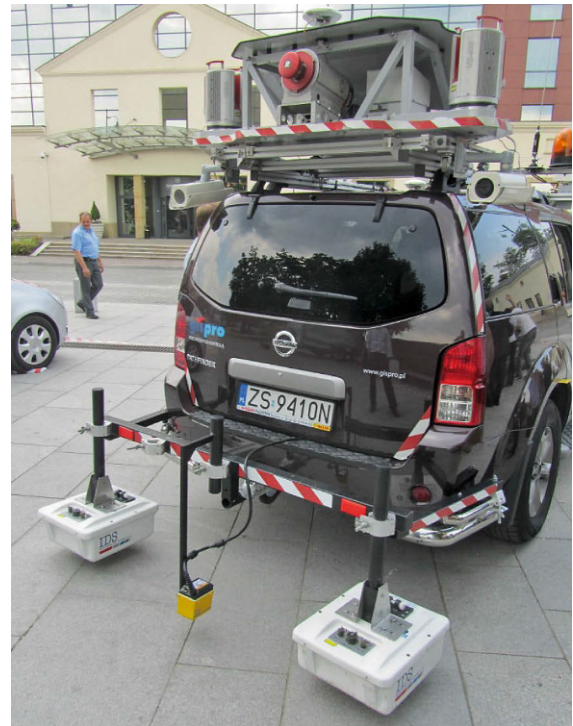
Fig. 35.14 Mobile mapping system (MMS) installed on a road vehicle. The system comprises multiple imaging sensors (cameras pointing forward, sideways, and backward), a laser scanner (on the top of the vehicle), a GNSS antenna (at the top of the van), and an inertial navigation system for platform orientation (box on rack next to laser scanner). Note also that this particular MMS is carrying additional sensors (mounted low to the ground) for radar imaging of the road surface and detection of cracks in pavement (courtesy of Charles Toth)
