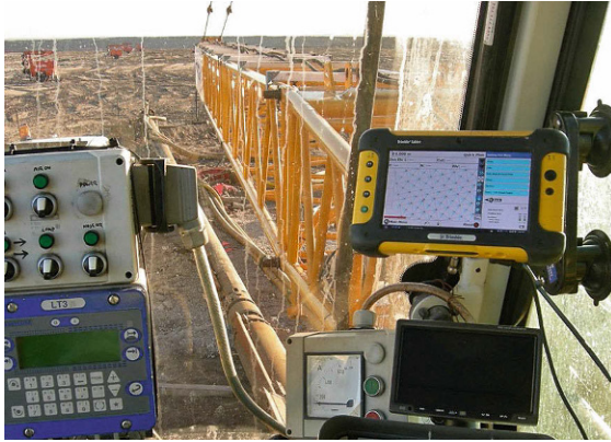
Fig. 35.13 Inside cabin of GNSS-assisted machinery – one or more GNSS receivers/antennas (multiple antennas provide vehicle orientation information) are installed on construction machinery and real-time solutions for position (and perhaps orientation angles) of the reference point on the vehicle are displayed to the machinery operator on a controller device together with the planned trajectory of the machinery so that the excavation may be carried out according to design (courtesy of Ultimate Positioning)
