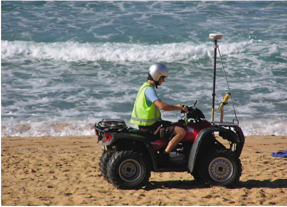
Fig. 35.3 Precise kinematic GNSS survey: the receiver is installed on a quad-bike with the antenna mounted upon on a pole, and the kinematic positioning task consists of determining coordinates of the antenna on a continuously sampled basis (e.g., once per second) as the bike as driven up and down the beach, to determine a dense network of heights with centimeter-level accuracy for beach erosion studies; note that the antenna height must be corrected for the fixed height of the top of the pole above the ground level (courtesy of Brad Morris)
