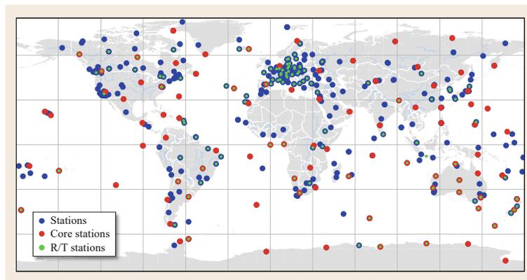
**Fig. 33.2** Sites in the global IGS tracking network. Out of an overall set of about 470 stations available in Oct. 2015, the 90 core stations marked in red are used to establish the IGB08 reference frame. Green dots indicate stations with real-time data transmission capability
