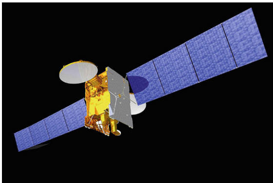
Fig. 12.4 The ANIK-F1R GEO used by WAAS (reproduced with permission of the the FAA satellite navigation team)
