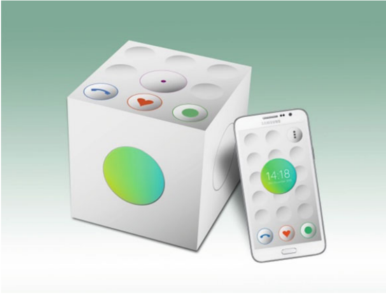
Fig. 2.3 User interface of the system consisting of a cube shaped object with a “Wellbeing state” indication (dynamically lit area in front). On top of the cube there are 3 lens-shaped tags for messaging. Next to the cube is a smartphone running the RelaxedCare-App. Source RelaxedCare Consortium, Ralph Eichenberger Szenografie
