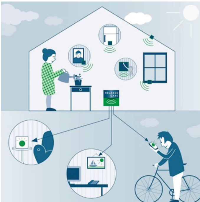
Fig. 2.4 System architecture. Sensors in the house of the AP are connected to the smart home server. The resulting wellbeing status (WBS) is shown to the IC via objects (cube, picture frame), or app. Source RelaxedCare Consortium, Ralph Eichenberger Szenografie
