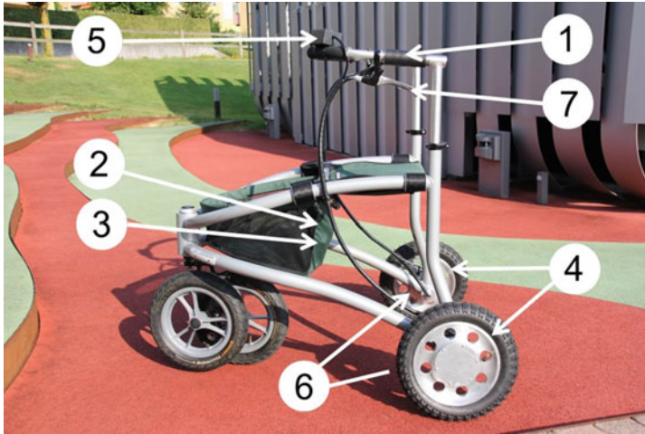
Fig. 2.9 The Active Walker with the major components of the e-Drive indicated. Source iWalkActive Consortium, iHomeLab
