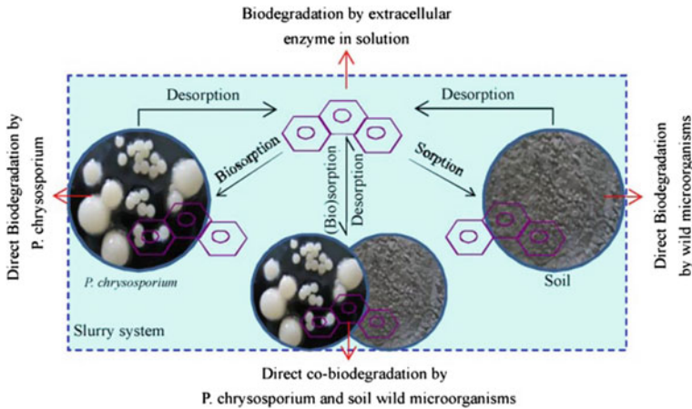
Fig. 4.8 The schematic diagram of (bio)sorption and biodegradation processes of PAHs in soil slurry systems containing Phanerochaete chrysosporium (Chen and Ding 2012)
