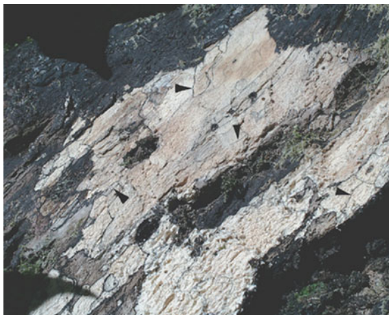
Fig. 5.3 Photograph of wood attacked by a white-rot fungus. Source www.bio.miami.edu/dana/pix/whiterot.jpg
