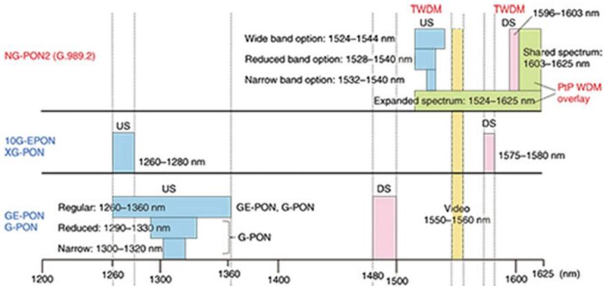
Fig. 9.7 Wavelength allocation plan for PON standards for backwards compatibility
