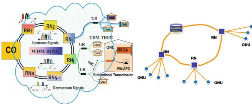
Fig. 9.5 Implementation of hybrid WDM-TDM-PON networks in the ACCORDANCE project [20]
