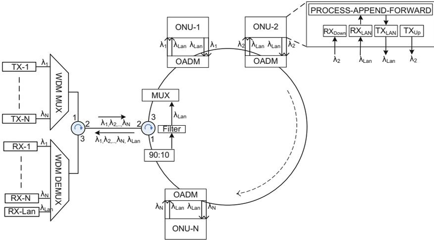
Fig. 9.8 Ring-based C/DWDM-PON architecture [32]
