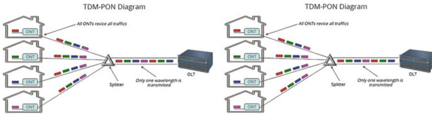
**Fig. 9.2** Time-division-multiplexed passive optical network architectures
