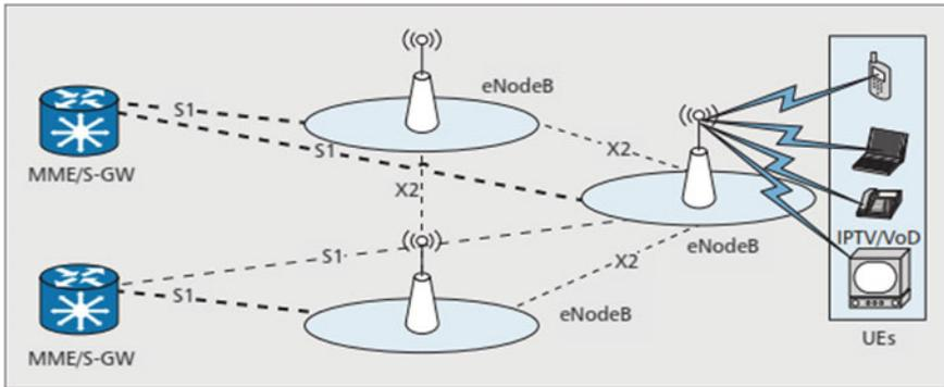
**Fig. 9.1** LTE network architecture
