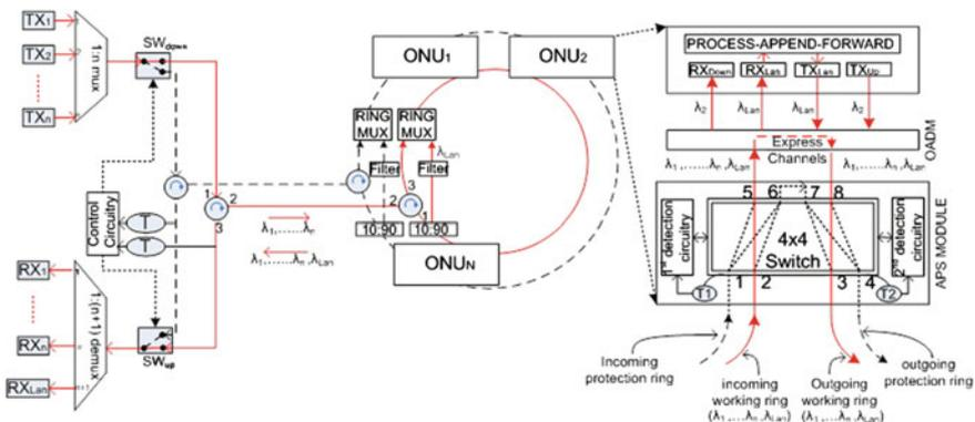
Fig. 9.9 Self-healing ring-based C/DWDM-PON architecture [38]
