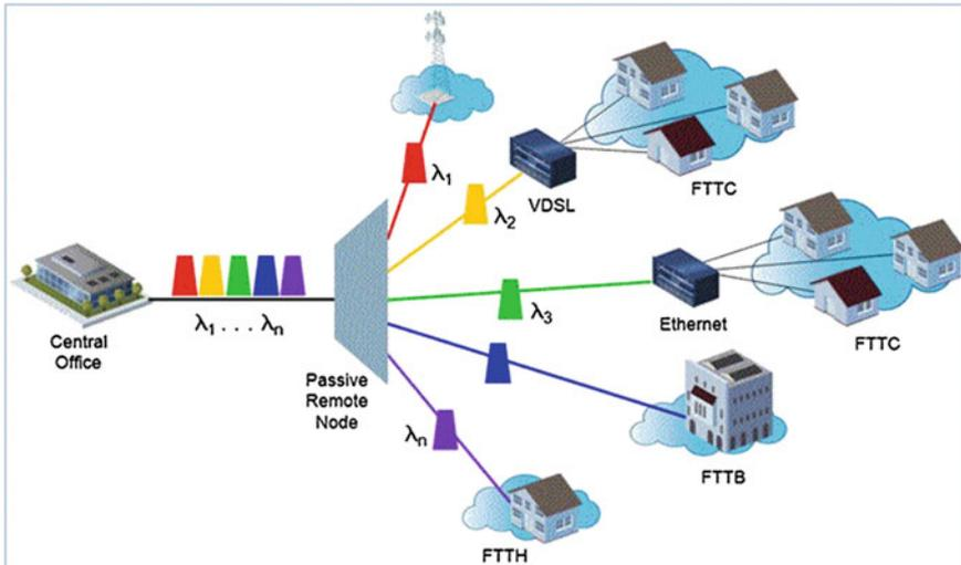
**Fig. 9.3** Wavelength-division-multiplexed passive optical network architecture
