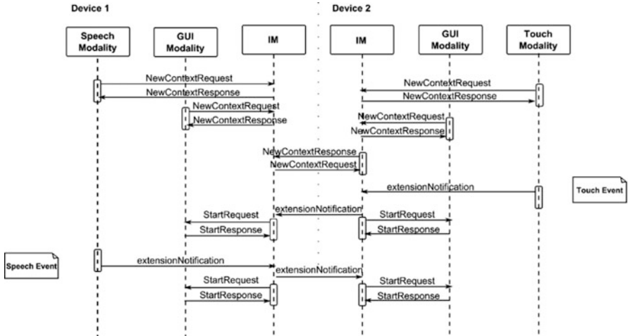
Fig. 17.3 Illustrative example of the communication between components for an MMI multi-device scenario. The touch and speech events, issued on one of the devices, are propagated to the other device through the Interaction Managers
