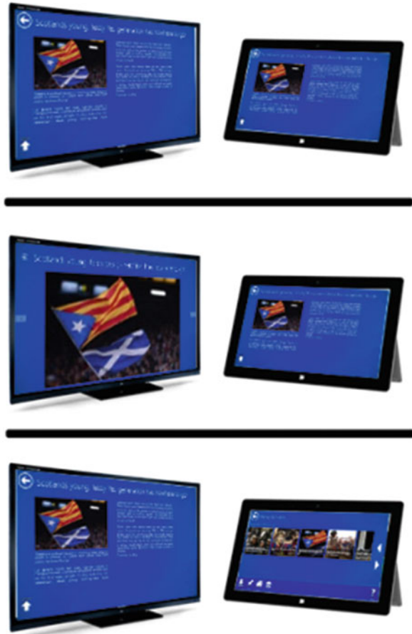
Fig. 17.6 Multiple ways to present the information available for a news content in a multi-device scenario including a TV and a tablet. From top to bottom : (a) both devices show the same content; (b) the TV shows a large image and the tablet the complete news contents; and (c) the TV shows the complete news contents and the tablet shows a news navigation menu
