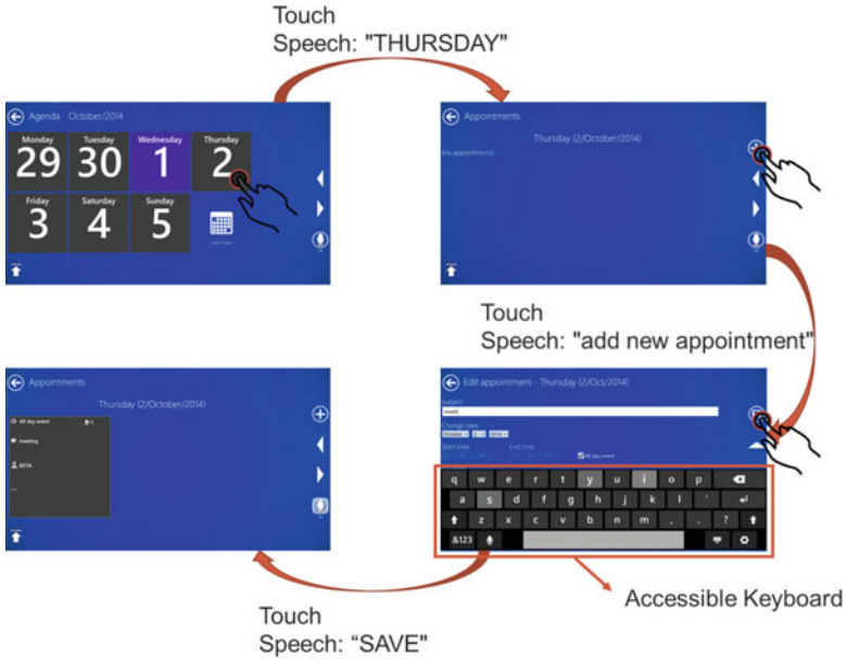
Fig. 12.8 Interactions flow to create a new appointment in the agenda, the user starts by choosing the preferred way to interact with the application (touch or speech) to select the day and then select the option to add a new appointment, then fill the subject with the virtual keyboard, and again select to save the appointment by touch or speech
