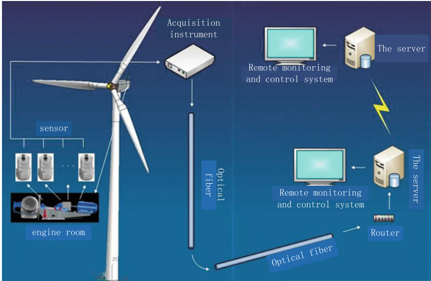
Fig. 27.2 Condition monitoring and fault diagnosis system of large scale wind turbine
