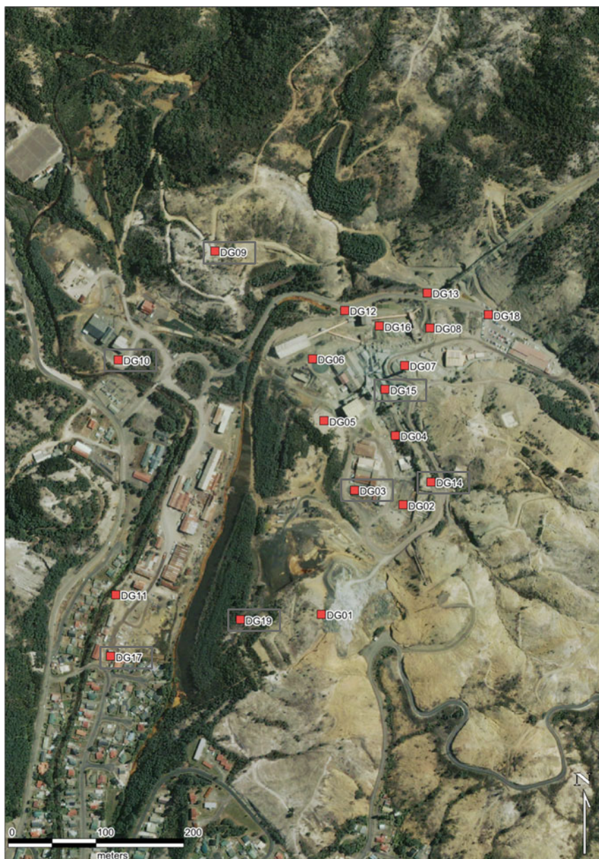
Fig. 2 Location of dust deposition gauges at the Mount Lyell mine site. The samples used in this study are highlighted in grey boxes . Source Copper Mines of Tasmania (Color figure online)
