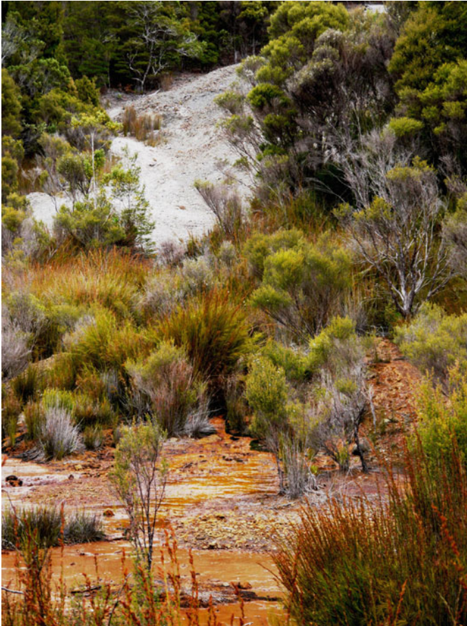
Fig. 3 ARD affected stream and historical waste rock piles at the Spray mine, Zeehan Field, western Tasmania (color figure online)
