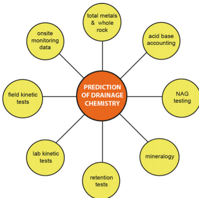
Fig. 1 The 'wheel' approach for predicting drainage chemistry (Morin and Hutt 1999). (Reprinted from Morin KA, Hutt NM (1999) Kinetic test and risk assessment for ARD. In: Proceedings of the 5th annual BC metal leaching and ARD workshop, Vancouver, pp 1–10, with permission from K Morin) (color figure online)
