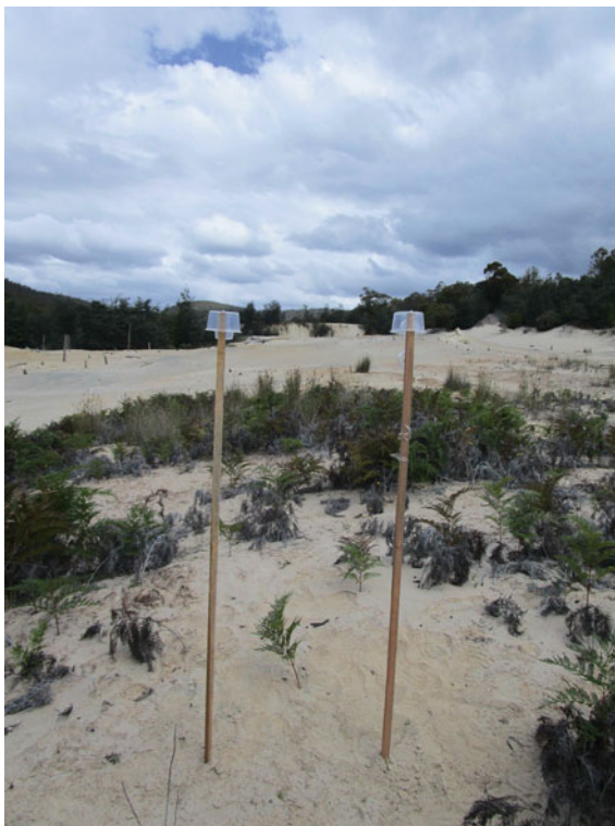
Fig. 6 Site PDS-1 with dust sampling devices deployed in the field for one month, Mathinna tailings dump. Dust sampling devices are \sim 1.7 m above ground (color figure online)
