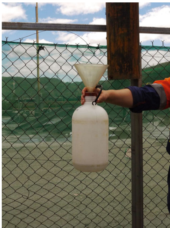
Fig. 3 Dust deposition gauge with stand (DG18)
