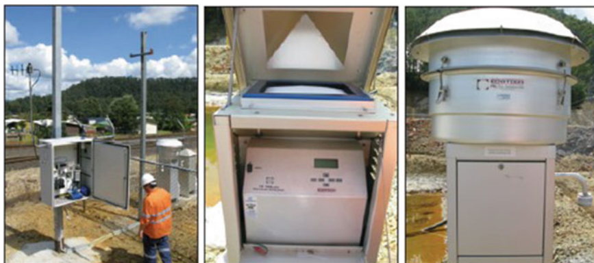
Fig. 1 Two high volume air samplers monitoring TSP and PM 10 at an offsite location near a mine ( left ). Close up of the filter paper shown under the lid of the TSP sampler ( centre ). The PM 10 high volume sampler situated adjacent to the TSP sampler ( right ) (color figure online)
