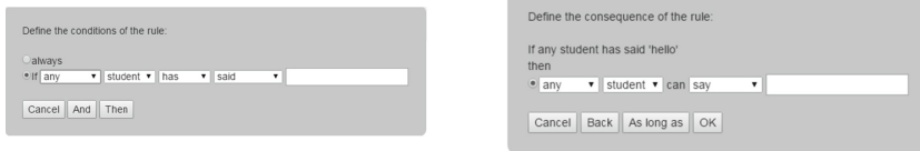
Fig. 1. Two screen shots of the SIMPLE editor. Users write sentences simply by selecting available options, and they can only write free text whenever the syntax rules indeed allow that. Therefore it is impossible to write malformed sentences.
