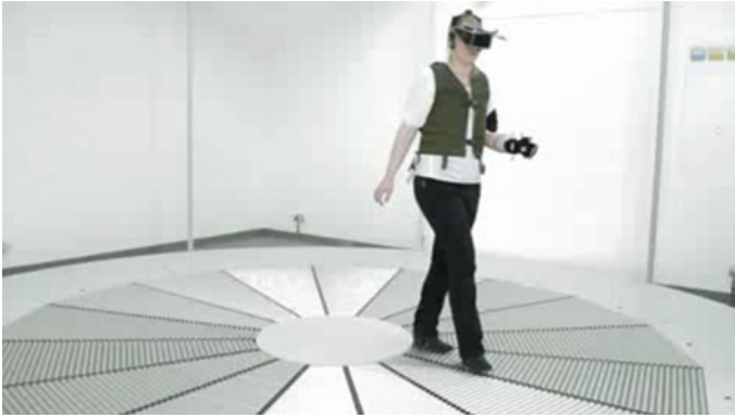
Figure 3 A test-person walking through a virtual world on the ‘Virtual Theatre’
