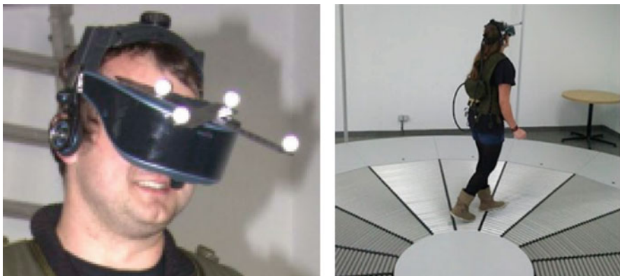
Figure 4 Head Mounted Display and omnidirectional floor of the Virtual Theatre
