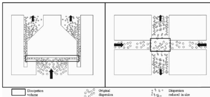
Fig. 4.17 Basic homogenization principles: piston gap ( left ) and jet-stream arrangement ( right ). In the piston gap homogenizer the macrosuspension is forced to pass through a small gap (few microns), and particle breakage is due to shear forces, cavitation, and impaction. In jet-stream homogenizers the collision of two high-velocity streams leads to particle breakage mainly by impact forces (Adapted from Muller et al. (2006))
