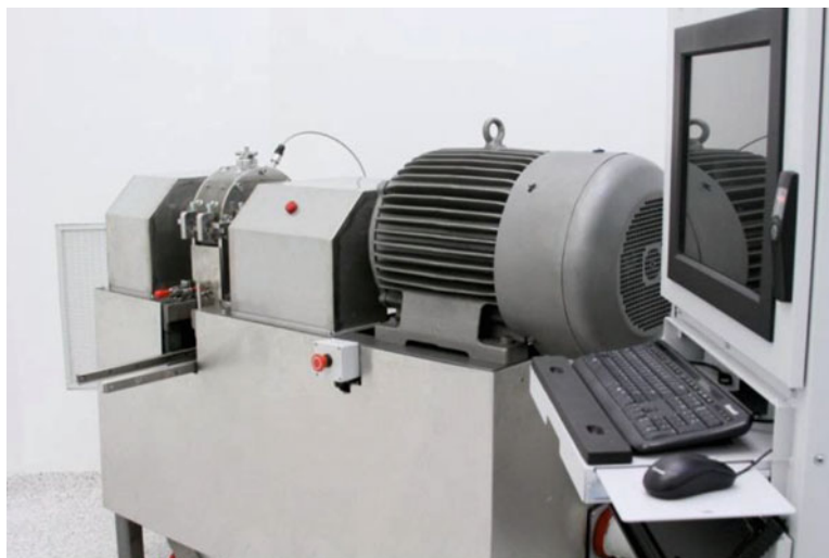
Fig. 13.2 Kinetisol® KC254B Compounder for batch-mode operation (Courtesy of Dispersol Technologies)
