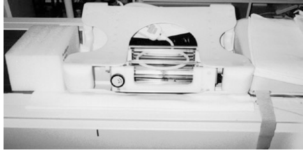
Fig. 12.2 An image showing a breast biopsy compatible MRI coil
