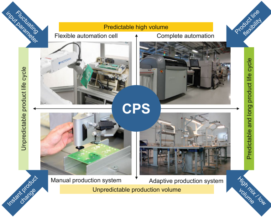
Fig. 3 Flexible production at mass-production efficiency enabled by CPS
