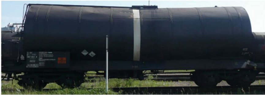
Fig. 1 Tank wagon for the transport of liquid petrochemical products [14]
