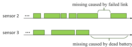
Fig. 1. Illustration of the continuous data missing in a dataset whose data points are returned by two wireless sensors
