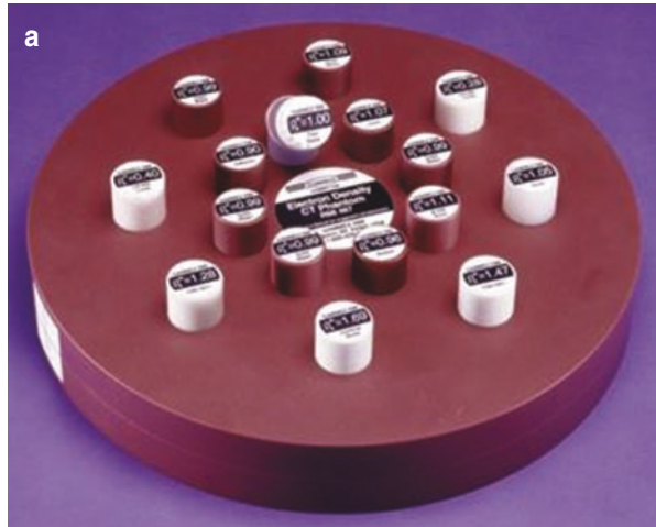
Fig. 3.6 (a) Gammex tissue characterization phantom. (b) Arrangement of tissue substituting rods (Courtesy of Sun Nuclear)
