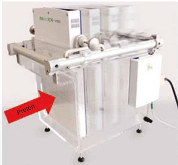
Fig. 2.11 Setup photo of DigiPhant with beam coming from the left ( red arrow ). The detector array automatically stops and acquires data at multiple programmed locations within the water tank during measurements (Permission pending IBA dosimetry)
