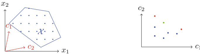
Fig. 1. Feasible space of a bi-criteria integer maximization problem and corresponding set in objective space with dominated points (blue), supported non-dominated points (red) and unsupported non-dominated point (green) for a maximization problem. (Color figure online)
