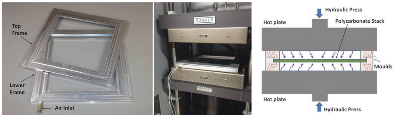
Fig. 6.5 Aluminum frame (left) to hold polycarbonate stack in hot press (center), and a side view schematic of the polycarbonate stack in the molds within the hot press (right)
