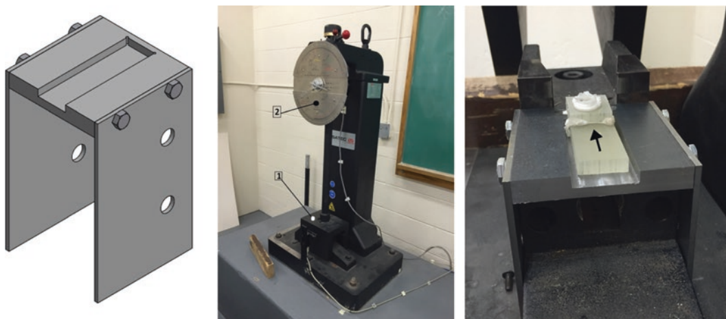
Fig. 7.4 CAD model of impact test rig, isometric view (left), the thickness of side walls are 3.175 mm, the Instron SI-1D3 impact tester (center), and test rig with mounted impact sample (right). The direction of the striker is shown by the arrow
