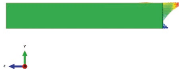
Fig. 7.9 Stresses in z direction plotted on the y - z cross section. Arrows in the negative z -direction are tensile stresses, arrows in the positive z -direction are compressive stresses, and the thickness of material is 6.35 mm
