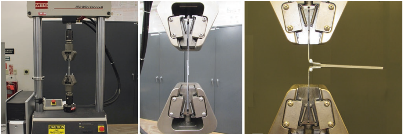
Fig. 6.2 MTS Mini Bionix II with lap shear sample (left), and close up of the lap shear test (center) and peel test (right)
