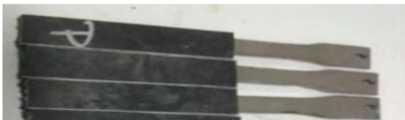
Fig. 12.2 Photograph of composite material bonded to truncated metal dogbone specimens for shear loading
