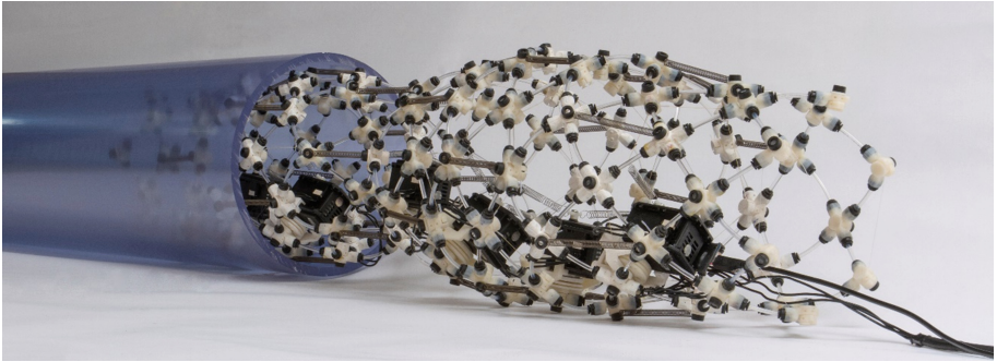
Fig. 1. The six-segment Compliant Modular Mesh Worm (CMMWorm) robot crawling through a 20.3 cm inner diameter pipe. The linear springs that passively return the robot to its maximum diameter are visible along the length of each segment.
