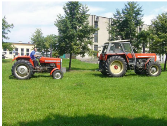
Fig. 3 Tractor unit URSUS 1204 during testing the measuring apparatus on the deformable pavement
