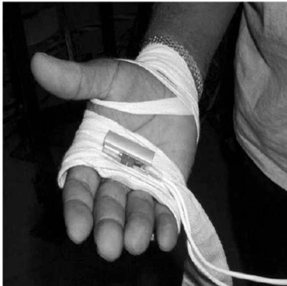
Fig. 2 Accelerometers in the palm of a boxer
