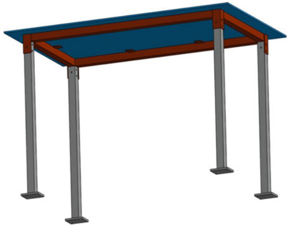
Fig. 2 Physical model of the adopted column-beam-plate system
