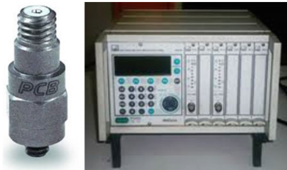
Fig. 8 Piezoelectric sensor and HBM measurement amplifier
