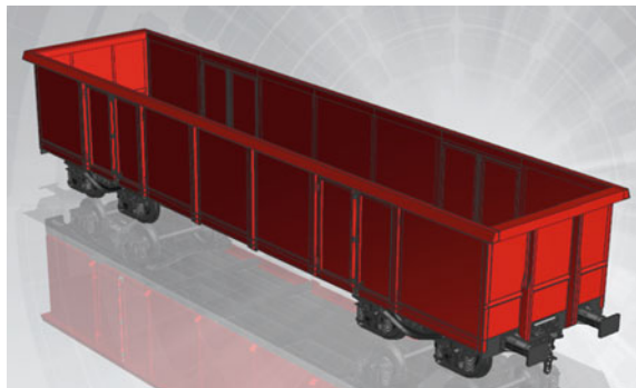
Fig. 1 The CAD model of the considered 4-axle open wagon series EAOS type 1415 A3
