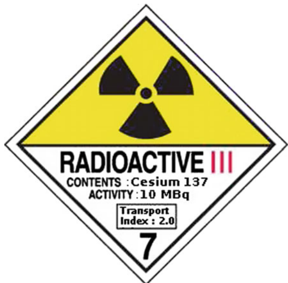
Fig. 12.1 Example of a label for a transport container, showing its radioactive inventory: it contains transport material of safety category III (in red letters), specifically the isotope ^{137}\text{Cs} , an emitter of both \beta s and \gamma s, with an activity of 10 MBq. The transport index 2.0 indicates a maximum dose rate at the surface of 2.0 mSv/h, and the number '7' refers to a wider system, in which radioactive material is class 7
