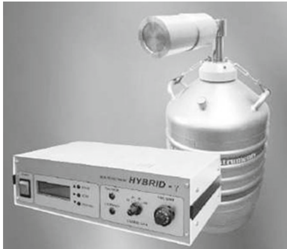
Fig. A.4 A germanium detector. The germanium crystal is the flat circular plate, and the flask underneath the detector (called a dewar) contains liquid nitrogen for cooling. (Image credit: NATS, Connecticut, USA, nats-usa.com/high-purity-germanium-planar-spectroscopy-system )
