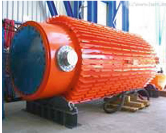
Fig. 12.2 CASTOR-like transport and intermediate storage container for spent fuel elements. (Image credit: www.bam.de )
