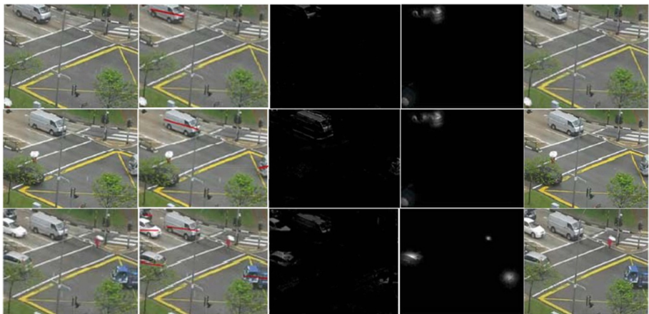
Fig. 4. increasing numbers of moving objects in dynamic scene. (a) input image. (b) moving cars detected by LIDAR. (c) map moving objects to grey image. (d) the method of Chen [6] in separating moving objects from the scene. (e) our proposed method in removing rain.
