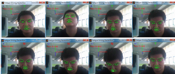
Fig. 9. We judge the fatigue driving state by the range of head pose, where Y represents the normal state, N represents the fatigue driving state.
