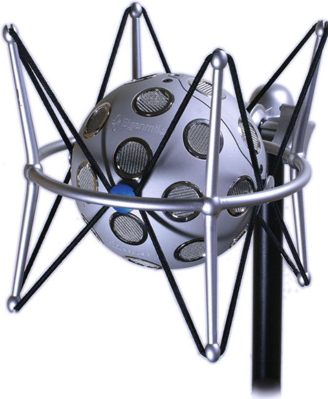
Fig. 1.2 The em32 Eigenmike spherical microphone array. This rigid array of radius 4.2 cm is comprised of 32 omnidirectional microphones. Copyright © Emanuel Habets. Used with permission
