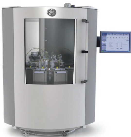
Fig. 13.42 SpinLab polarizer ( left ) and fluid path ( right ). The polarizer consists of a 5 T superconducting magnet and cryostat. The cryostat has a sorption pump that can drive the temperature of a helium bath to <0.9 K. The sample is irradiated with microwaves at 140 GHz. The polarizer has four channels that allow individual loading of the fluid path to the right. The fluid path consists of a
