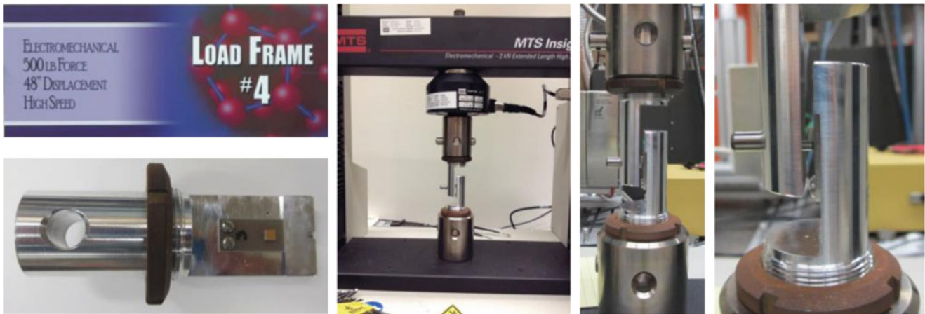
Fig. 12.3 Shear test apparatus and specimen mounted and tested in an MTS load frame
