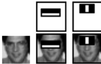
Fig. 10. Two features shown in the top row and then overlaid on a training image in the bottom row. The first feature measures the difference in intensity between the region of the eyes and a region across the upper cheeks. The second feature compares the intensities in the eye regions to the intensity across the bridge of the nose [6].
