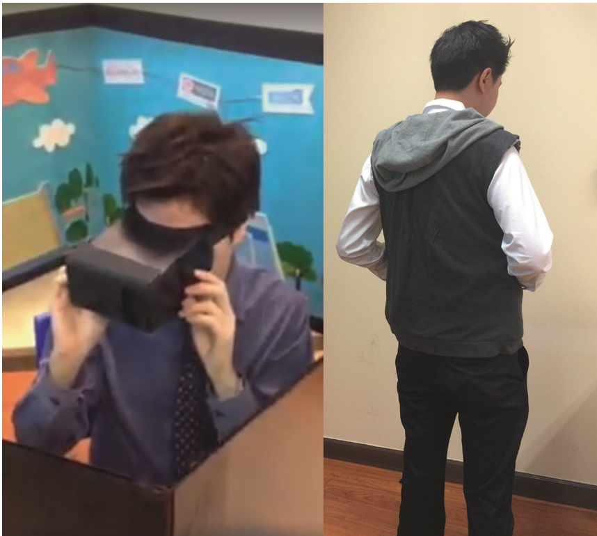
Fig. 4. A cardboard headset we created and integrated for allowing people with special needs to have an immersive experience about the scene and story using augmented reality technology and our extended wearable T.Jacket
