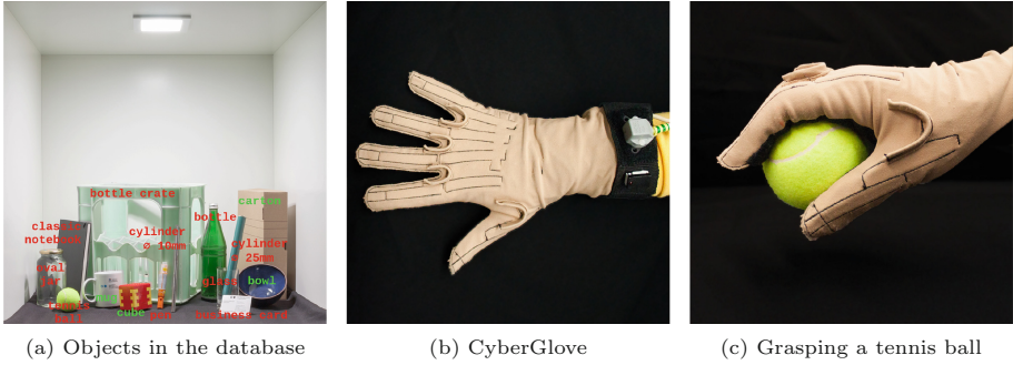
Fig. 1. (a) Objects used for grasping: classic notebook, oval jar, tennis ball, mug, cube, bottle crate, small cylinder, pen, bottle, glass, business card, bowl, cylinder large, carton ( 7.6 \times 26 \times 37.5[\text{cm}^3] ). Objects in red were used in controlled transport . (Color figure online)
