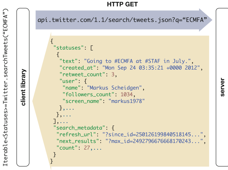
Fig. 1. Example request and response for a tweet search with Twitter’s REST API. The resulting JSON is simplified; strings are abbreviated.
