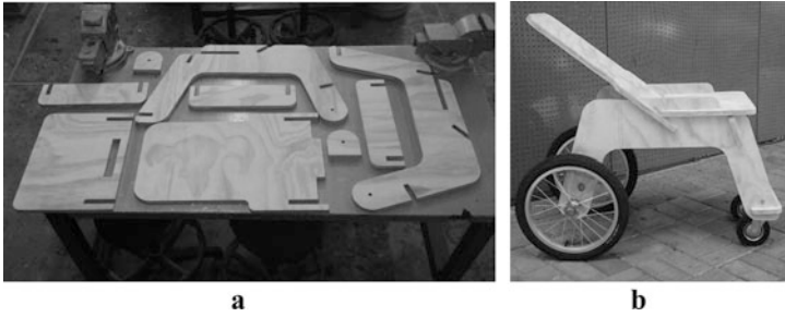
Fig. 7 a Pieces of plywood sheeting for a prototype. b Prototype ready for testing
