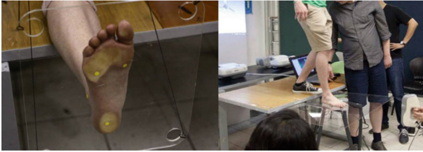
Fig. 4 Scanning and photogrammetry process. To produce scans of the foot under a load, loads were applied using a clear sheet of acrylic
