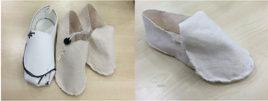
Fig. 3 Initial foam sheet and canvas material footwear soft goods prototypes based on the lasso shoes
