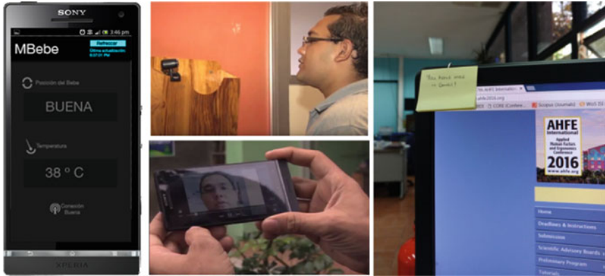
Fig. 4 Notification mechanism used in the four prototypes. Left “notifications for emergencies”—mobile application. Center “notifications for visitors in offices”—augmented door and mobile device. Right “notifications for particular emails and collaborative document editing”—post-it note placed in the work environment
