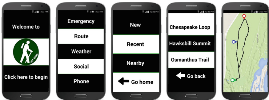
Fig. 3 Sequence of events for Task 3. Users select the bottom button to begin, select Route, and then select Recent. Next, they select Osmanthus Trail and access important trail information, such as shelters, water, or user-tagged hazards
