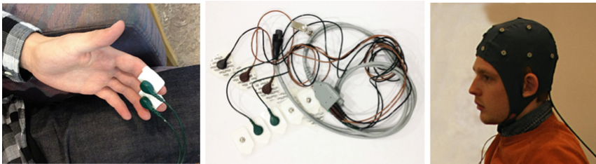
Fig. 2 GSR connections, ECG and EEG Cap, using 3 different solutions in the design lab to register emotional reactions of users
