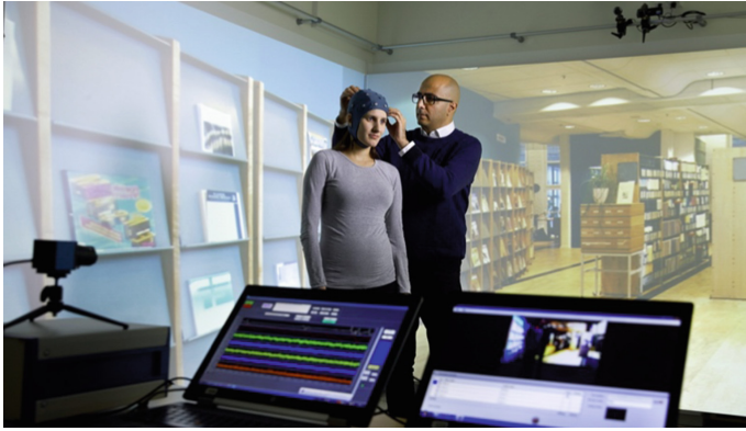
Fig. 3 Experimental set up, installing of EEG cap, ECG and GSR measurement tools and integrating with observation system in the design research lab
