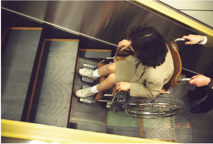
Fig. 5 An escalator with three steps flattened to accommodate a wheelchair. Compared to stair climber in Fig. 4, this does not allow frail seniors to use the system, thus they are excluded from being the users
