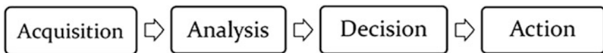
Fig. 1 Information-processing model. While this is a gross simplification of the complexity of human (or machine) information processing, it is useful in understanding the process of going from data acquisition to action execution
