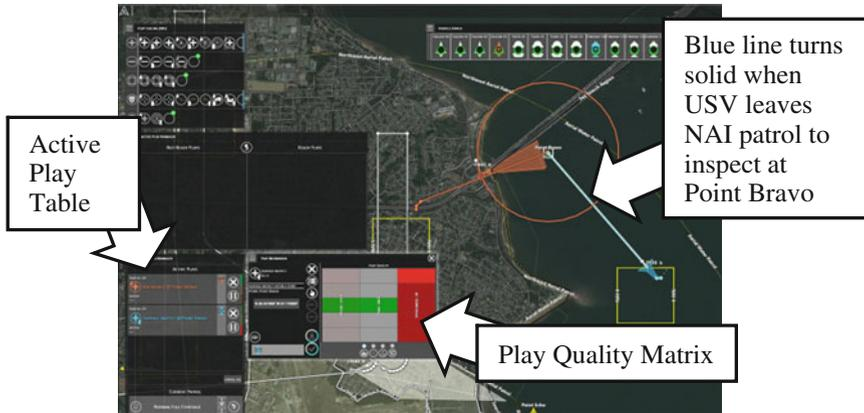
Fig. 8 Sandbox map showing both air and surface UVs on plays to inspect suspicious watercraft at Point Bravo and other UVs on normal full coverage patrol
