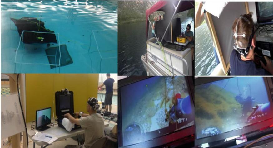
**Fig. 1** Video Ray Pro-III Submersible and B-Alert wireless EEG system worn by ROV operators supporting NASA's Pavilion Lake Research Project (shown during pool and field phases on the *left* and *right* respectively)
