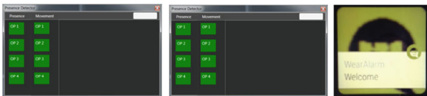
Fig. 3 HMI state 1.1 operator present, response supervisor PC, response operator PC, smartwatch
