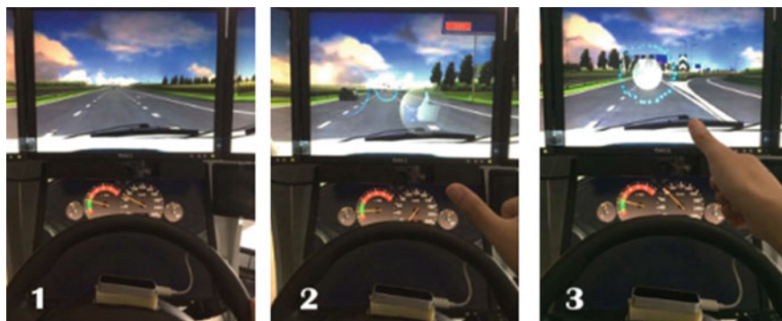
Fig. 5 Providing feedback to fellow drivers. Panel 1 The setup, showing a Leap motion sensor for gesture recognition. Panel 2 Making a thumb-up gesture to express “Like”. Panel 3 Selecting the recipient vehicle of the “Like” gesture through a pointing gesture
