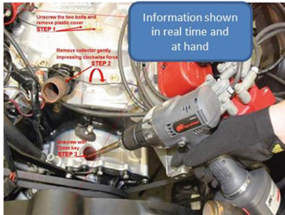
Fig. 8 AR showing procedural steps during on-board training as well as on-ground experts hints during remote support of ISS crew during malfunction operations
