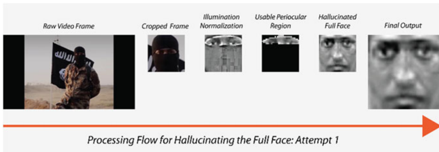
Fig. 11 Process flow for the reconstruction/hallucination of the full face of the suspect from just the sample video frame. The frame is first cropped and then de-rotated to obtain a near frontal orientation. Illumination normalization then helps in removing some of the effects of shadow. We identify a small usable periocular region which seems to contain the most amount of biometric identity. We then hallucinate the full face using DW-KSVD
