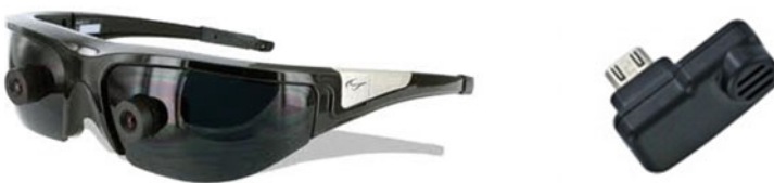
Fig. 4 Head mounted display and 6DoF gyros
