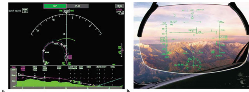
Fig. 1 Boeing 787 displays: a Navigation and vertical situation display; b HUD [4]
