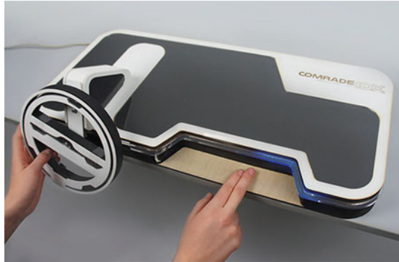
Fig. 2 The “Comrade” system, a tangible interface for negotiating control between driver and vehicle
