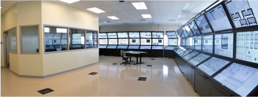
Fig. 1 The human system simulation laboratory (HSSL) with the generic pressurized water reactor control boards displayed on the three-screen bays
