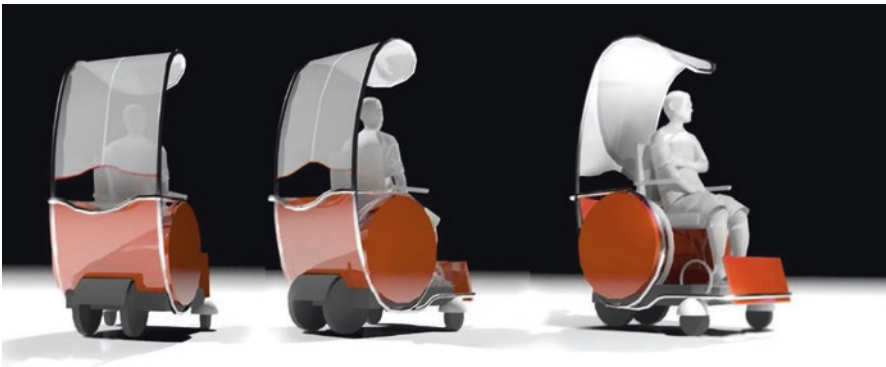
Fig. 6 Rendering of the concept version of the electrically powered transporter for persons with disabilities for the outdoor use. Solution has been declined due to the absence of front shielding (windscreen) (A. Bonenberg)
