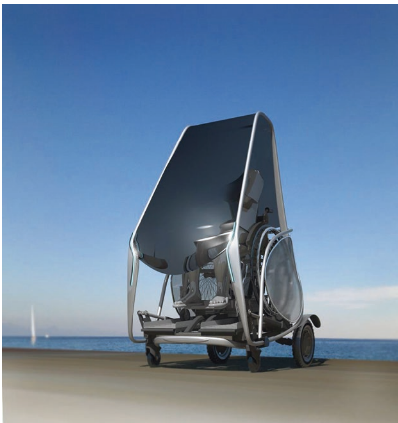
Fig. 1 Rendering of final form of the body of the electrically powered transporter for persons with disabilities, author: A. Bonenberg
