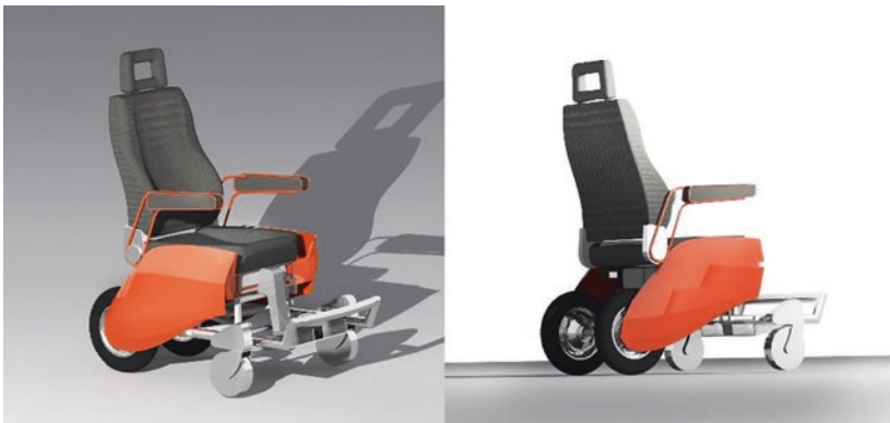
Fig. 3 Rendering of the final version of the casing of electrically powered transporter for persons with disabilities for outdoor use (A. Bonenberg)
