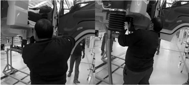
Fig. 5 Postures after the reduction of the cabin's height (operations previously performed under the cabin with the arms over the head)
