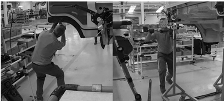
Fig. 7 Postures of the operator that shares the workstation after reducing cabin's height
