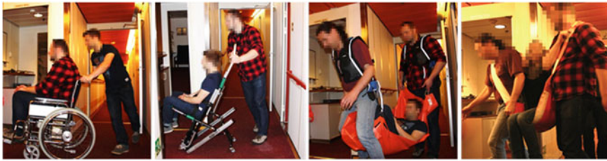
Fig. 1 Selected rescue devices in level condition; from left to right : standard wheelchair, rescue chair, rescue sheet with vest harnesses, and rescue seat
