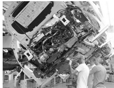
Fig. 2 Examples of operations performed with the arms above the shoulder line and with the torso side bend
