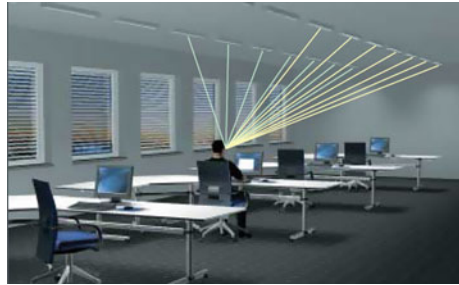
Fig. 8 Depending on the class of VDU, the mean luminance of luminaires which could be reflected on the screen needs to be limited to 200 cd/m 2 or 1000 cd/m 2 above a threshold angle of radiation of \gamma \geq 65^\circ (calculated at 15° intervals all around the vertical axis) to avoid disturbing reflections [14]
