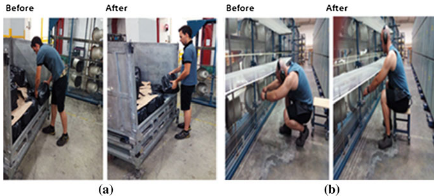
Fig. 5 Before/After implementation of a base of metal boxes (a) and a bench with wheels (b)
