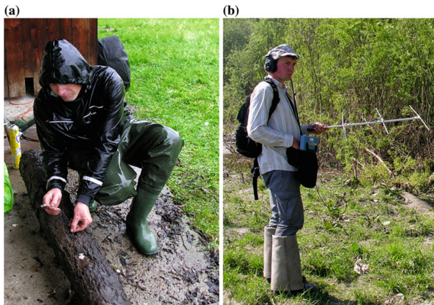
Fig. 8 a Installation of a radio transmitter in an alder log prepared for the tracking experiment. b Searching for the tagged logs after the flood of May 2014 using a TRX 1000WR signal receiver and a Yagi antenna
